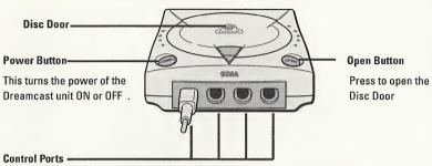
Use these ports to connect the Dreamcast Controller or other peripheral equipment. From left to right in order are "Control Port A", "Control Port B", "Control Port C" and "Control Port D". Use each port to connect controllers for players 1 to 4 respectively.
